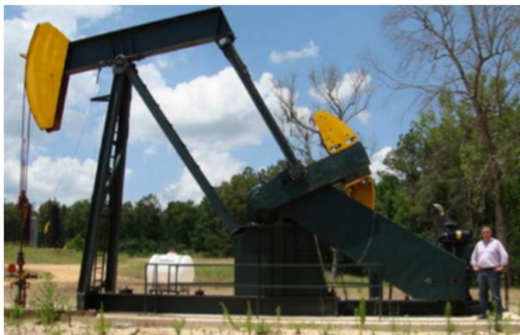
*Typical pumping unit on a Four Rivers well*
