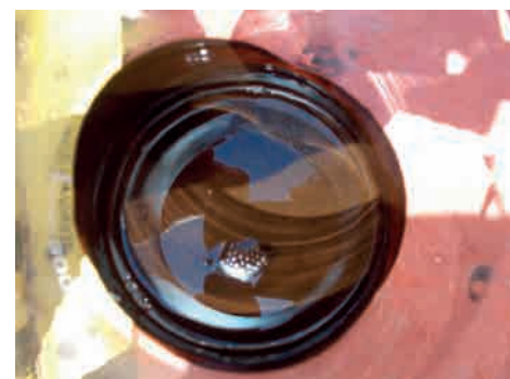
Baseline crude sample with Hydrocarbon Dynamics Multi-Flow at 40°C (400ppm). Baseline crude has a new Pour Point temperature of 32°C
